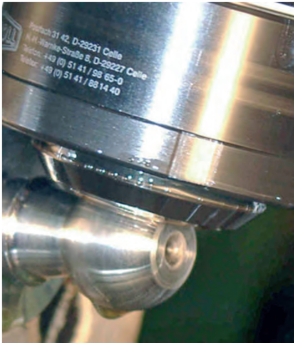
RKAK tool in operation
