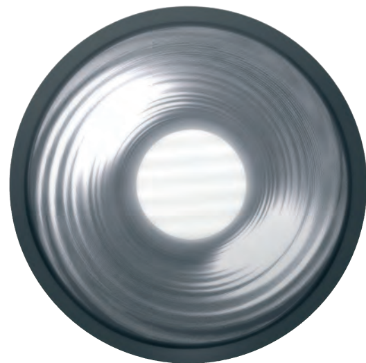
Cylinder with rippling problem
