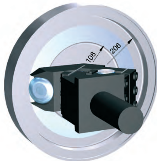
Machining a flywheel with an EG45-40M tool.
